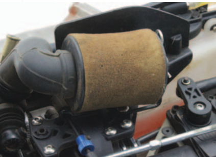
Even if the filter looks clean, it will benefit from a good cleaning. Don't forget that add some air-filter oil once it has dried!
