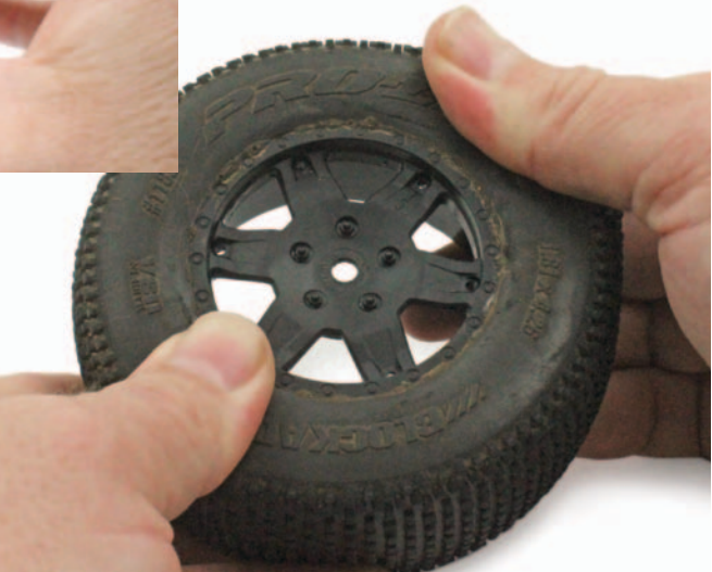
No matter how good your glue job is, you'll always want to give the tire a tug to make sure that it's still properly secured to the wheel.
