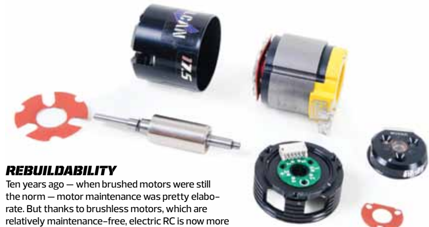
Disassembly of a rebuildable motor is easy — it's typically just a couple of screws!
