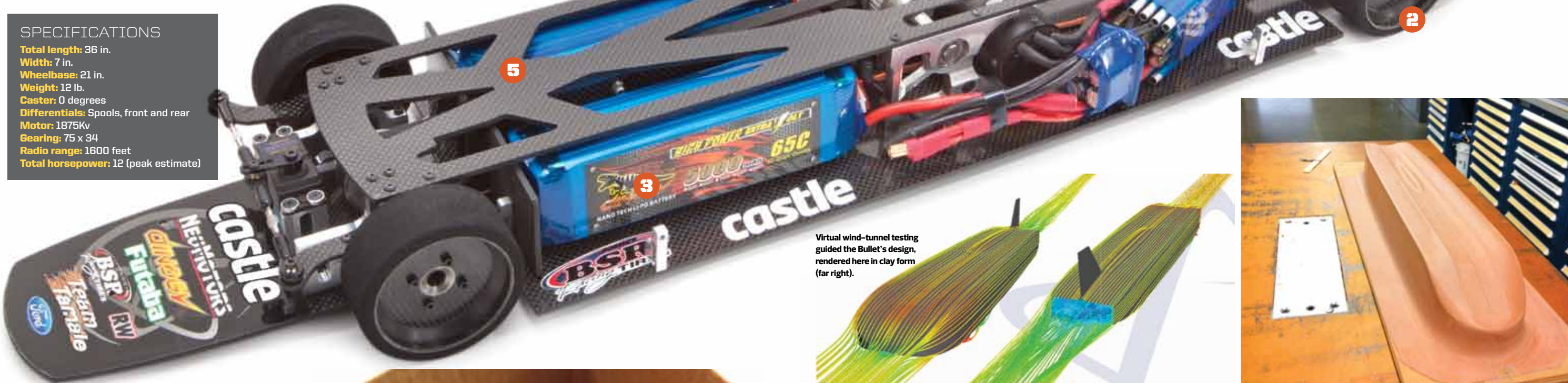
The wheels are constructed of rigid carbon fiber to run true at more than 20,000rpm.
