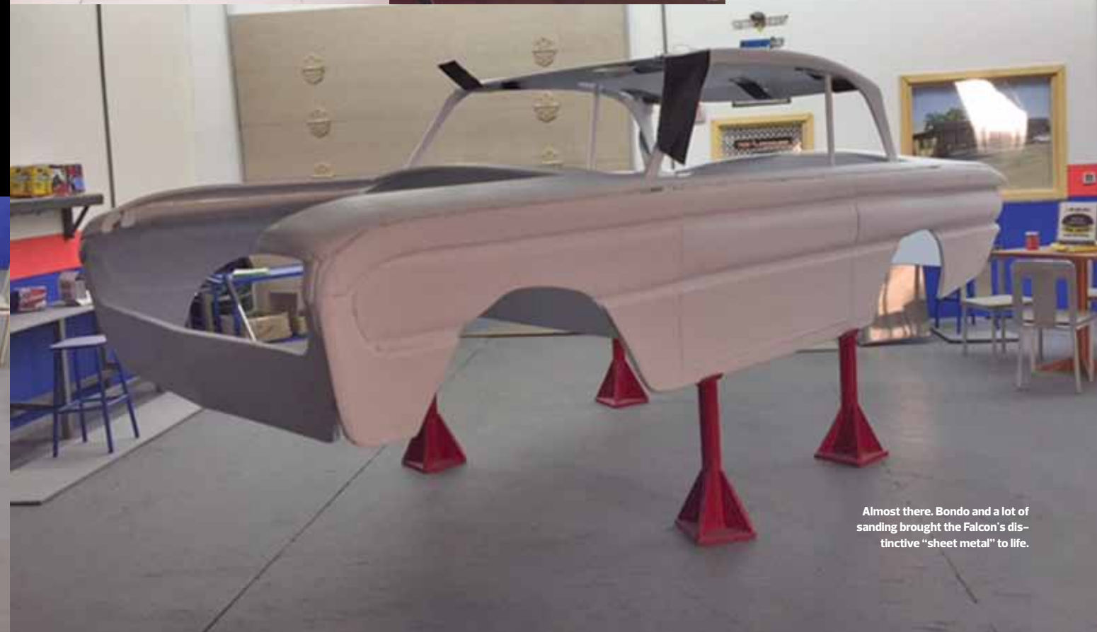
It's coming together. The shape is blocked out in sheet plastic.
