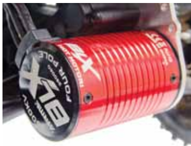
The included 80amp speed control is waterproof and spins a powerful 3600Kv 4-pole brushless motor.
