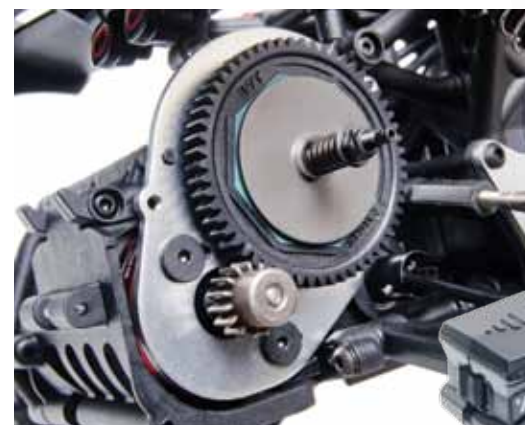
Like a 1/10 buggy, only bigger. The Raider XL pairs 32-pitch gears with a dual-pad slipper clutch for maximum durability.
