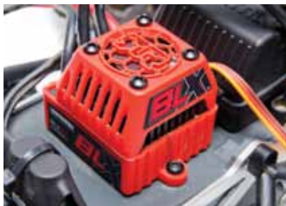
The included 80amp speed control is waterproof and spins a powerful 3600Kv 4-pole brushless motor.
