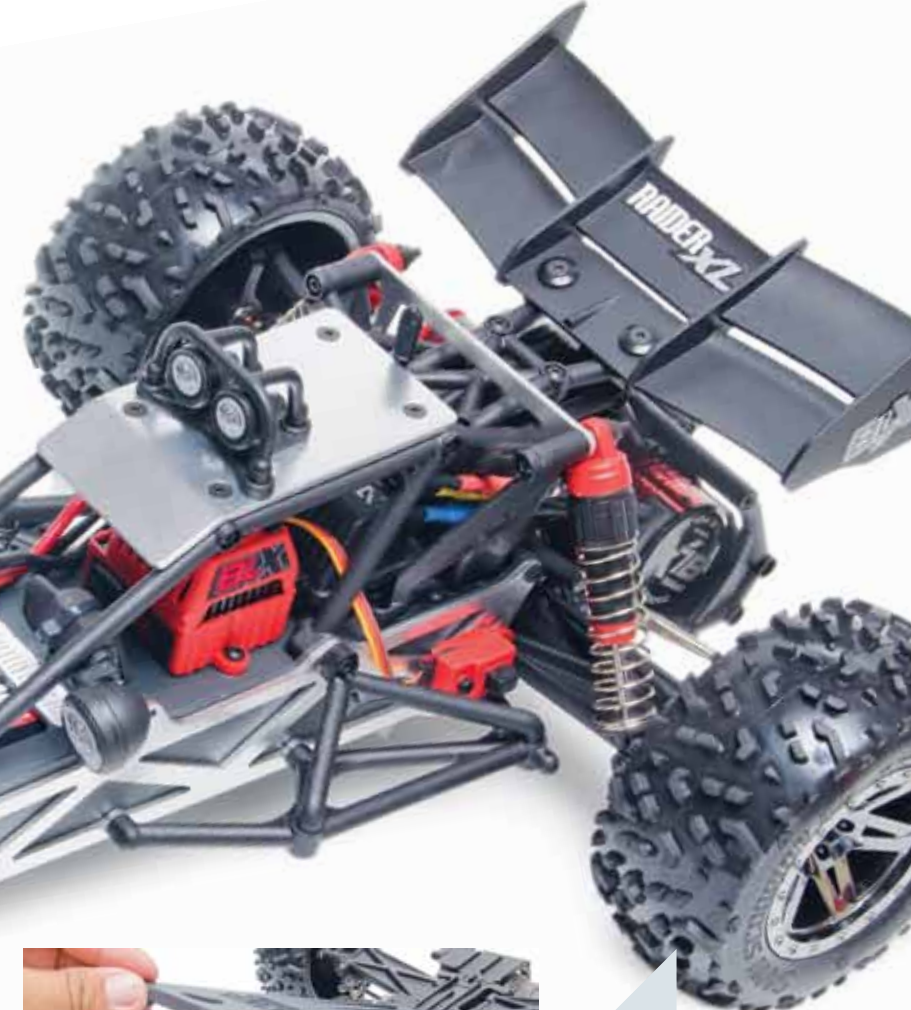
dBoots offers a full line of race treads, but the Raider's dBoots rubber is definitely designed for fun with an all-terrain tread design and firm compound that should offer long wear.
