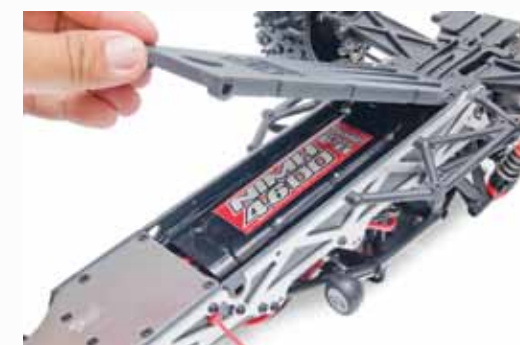
Removing a pin lets you flip open the chassis' underside for quick battery changes.
