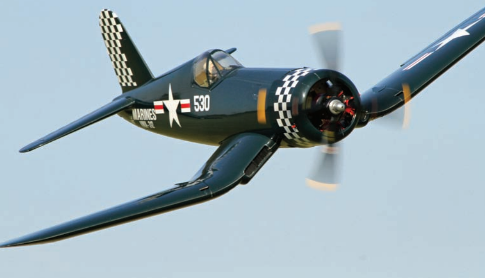
Piloted by Dennis Shrewsbury, this Composite ARF Models 110-inch-span model is powered by a Hacker A200 motor spinning a 28 x 14 prop with 14S LiPos (two 7S packs in series).
