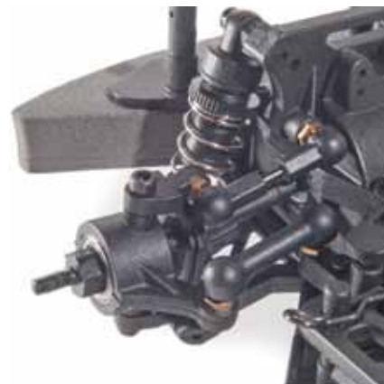
The steering links are fixed-length, but camber is adjustable. Ball bearings are standard, and the wheels slide onto 7mm hexes.
