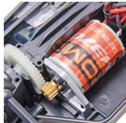
As seen here on a brushed model, a metal motor plate draws heat away from the motor and keeps the mesh from drifting.
