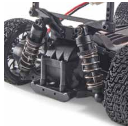
Oil-filled shocks smooth the ride. The plastic bodies are threaded for easy preload changes.
