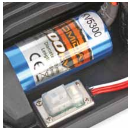
This little blue bullet is good for 27mph on the included NiMH battery. The electronics are waterproof; note the silicone-covered switch.
