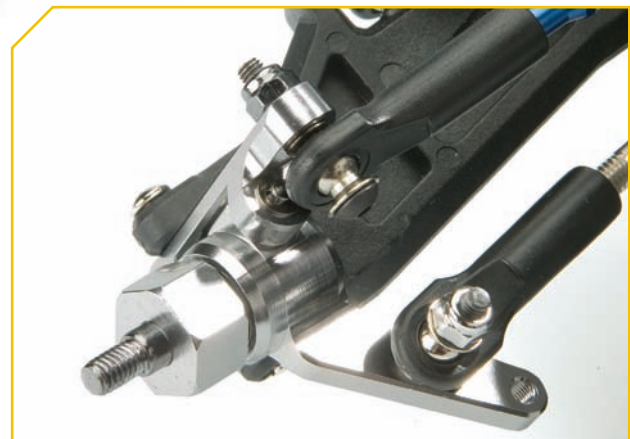
The jewel-like caster blocks and steering blocks are direct fits, and they substantially increase durability.
