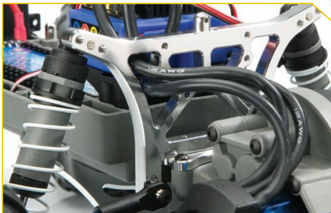
The rear shock tower has plenty of room to route the motor leads, and it is far more rigid than the stock tower.
