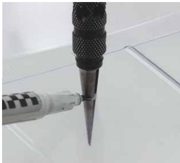
If your ream doesn't have marks on it, make one hole to the correct size, then place the ream back in the hole and mark it along the outside of the Lexan so you know where to stop.
