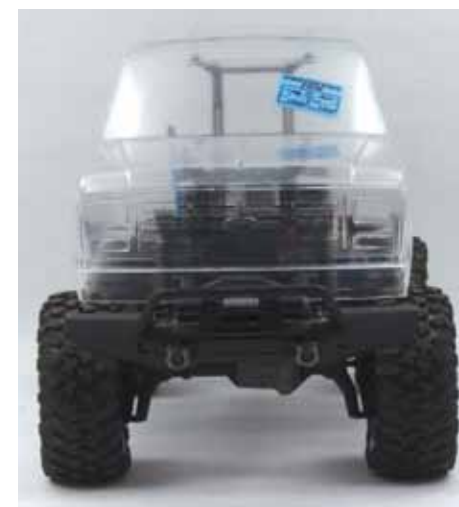
Align the body front to back, then side to side.
