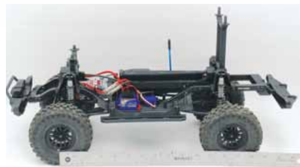
Measure the distance between the centers of the wheels to get the truck's wheelbase if you can't find the information online or in the manual.
