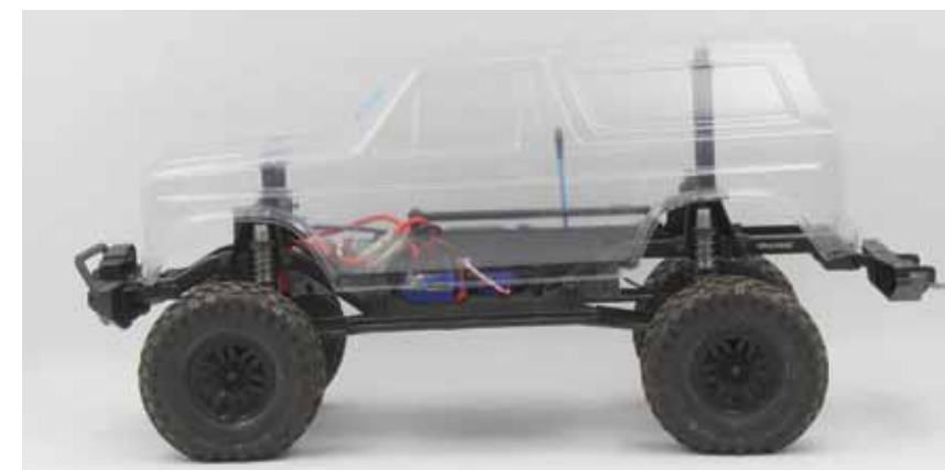
Adjust the body mounts so that the body sits level on the chassis before marking the post hole locations. If you leave it sitting at an angle like this, you may have post holes that are slightly off.
