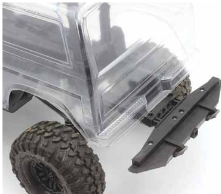
When getting the body to the right height on the chassis you may run into parts that interfere with it. You may have to trim the body to clear these parts.
