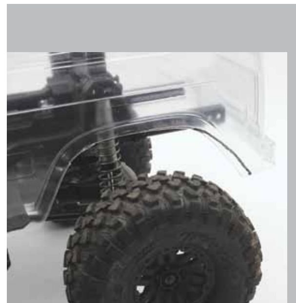
When you pick a body that doesn't have the same wheelbase as the truck that you're putting it on, you may have to trim the wheel wells slightly to make it fit better.
