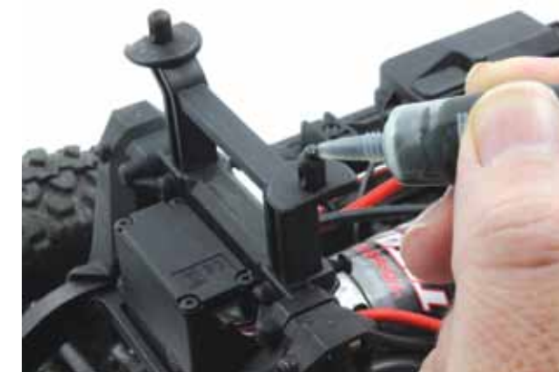
A little dab of grease is all you need to locate the body post on the bottom of a painted body.
