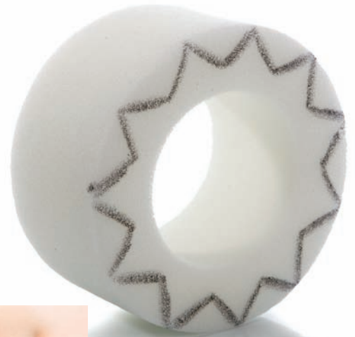
Above: cut your inserts in a star pattern to soften up the foams. This will allow the tire to conform to the rocks and still give it enough support. Left: memory foam is the latest trend in tire inserts.
