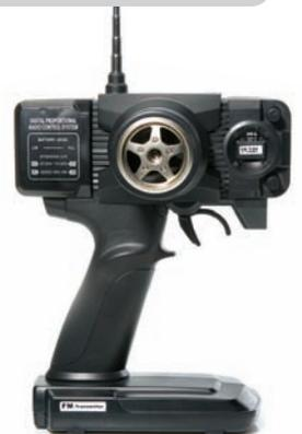
The included 27MHz FM radio was reliable during testing. EPAs, throttle/servo high/low and servo-reversing are all adjustable.
