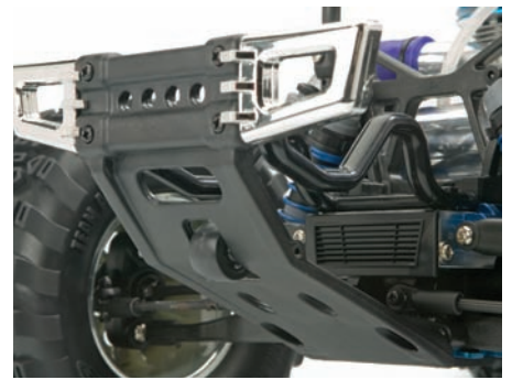
A small wheel is mounted in the rear skidplate to give the MGT 8.0 extra stability in wheelie mode.
