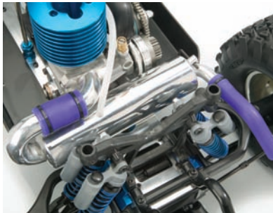
Big engine, big pipe. The long stinger keeps exhaust goo away from the tires.
