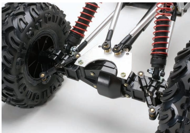
The rear suspension is a little less cluttered because it lacks a rear steer setup.
