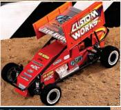
The Enforcer's body comes in pieces that, when assembler, make for one slick-looking, realistic sprinter. The two side panels have header-pipe details, and the left side has a molded-in starter motor. Zegers RC Graffixx did the painting, and I added the popular Custom Works Speedway hood to increase front downforce. Custom Works offers a ton of other cool bodies you can cheek out on its website.
