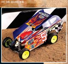
Many EDM racers carefully cut and fold sheet Lexan to make their own bodies, but McAllister Racing makes this far more rea tic (and convenient) shell. The side and roof sections are still made out of sheet Lexan, but the inner section is a more traditional cuum-molded piece. Zegers RC Graffixx whipped up the awesome paint job.
