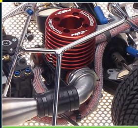
Fantom's FR12 rear-exhaust racing engine produces 1.15hp with a max rpm of 41,700. All in all, the FR12 is a nice-looking, powerful engine.
