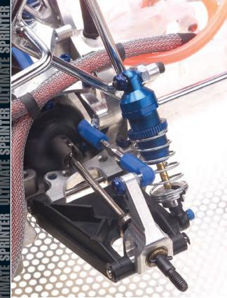
To achieve the right look and scale appearance, I installed wide-track Associated RC10 buggy A-arms. The rear arms are mounted on Hammad Ghuman aluminum GT zero-degree mounts. The titanium hinge pins and turnbuckles are from Lunsford, and they're paired with hardened-alloy ball joints from Hammad Ghuman and RPM's heavy-duty ball cups.
