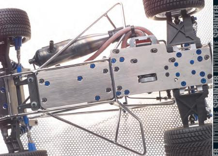
The Bullet frame is completed with a stock RC10GT chassis that must be cut follow-ing a template that's included with the tube frame. I skipped this step and instead gave the Ultimate Sprinter three custom titanium pieces cut by Hardcore Racing.
