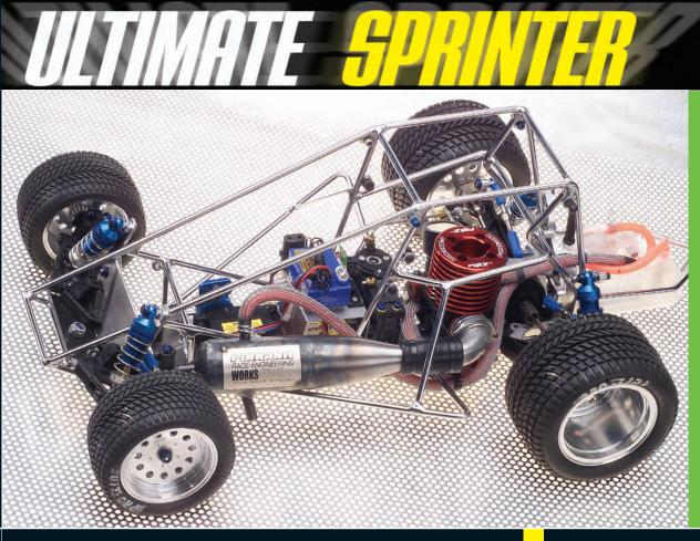
Bullet Racing out of Phoenix, AZ, produces a real "downtube-style" frame. Made of 5/32-inch high-tensile steel rod, it looks like the real thing, it's rugged and it's functional; all the welded joints are smooth, clean and nicely filled. Gussets are well placed in highstress areas. It's available in 20 powder-coat colors and two plating colors, so you are sure to find the color you want.
