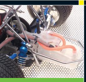
To hold everything together, I used Associated anodized hardware. The fuel lines and pressure tube are covered with electrical wiring nylon "snake" tubing and painted silver to imitate braided line. You have to remove the tail sec-tion frequently to access the fuel cell, so it's held in place by a standard post and body clip.
