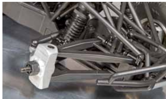
The plastic shocks feature threaded bodies for easy pre-load adjustment. The shock mounts are incorporated into the roll cage.
