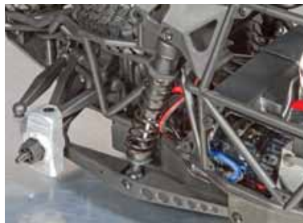
The rear suspension is not your typical lower A-arm setup seen in RC. A more realistic trailing arm design is used instead.
