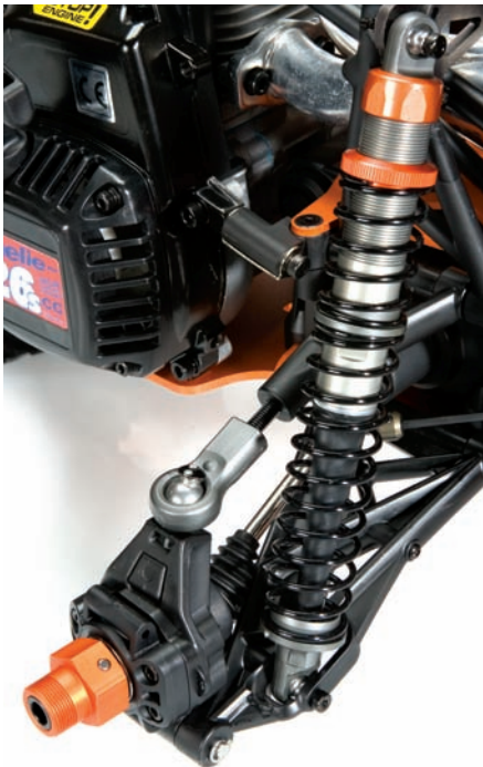
The shocks feature threaded bodies for easy ride-height adjustment, and the 6mm shafts are thicker than the RTR 5B's for increased durability.
